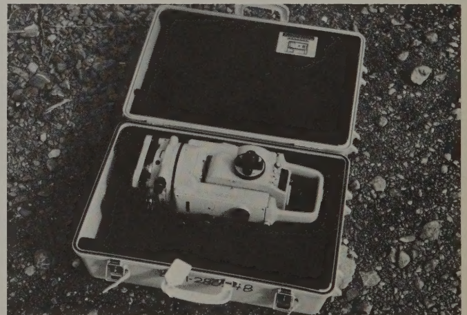
A total station for measuring both angle and distance between points.
